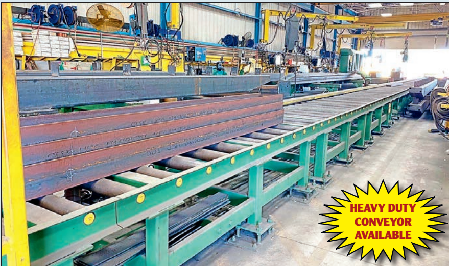
350' HEAVY DUTY ROLLER CONVEYOR LINE, 42" ROLLER CONVEYOR WIDTH, 350' ROLLER CONVEYOR LENGTH, 500 LBS./FT., WEIGHT CAP., (3) CONTROL STATIONS, (3) 5 HP HYDRAULIC MOTORS.
