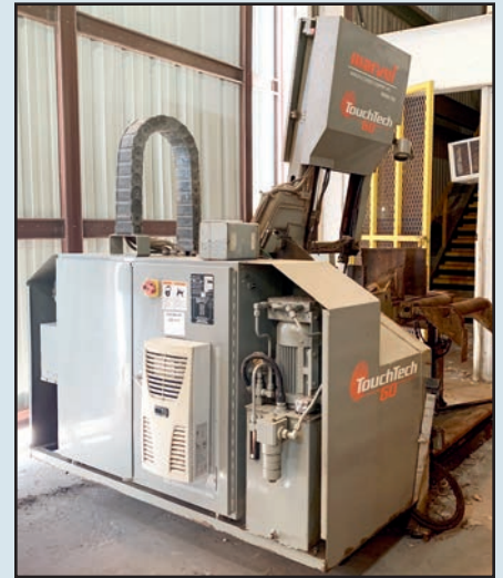
MARVEL F215010227TS HORIZONTAL BAND SAW, 20" X 25" CAPACITY 20" X 17" @ 45° CAPACITY, 30-650 FPM BLADE SPEED WITH INFEEED AND OUTFEED CONVEYORS.
