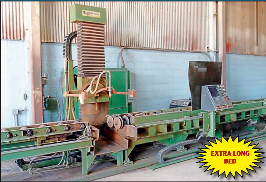
VERNON MPM4-0224 PROFILER, 60' BED, WITH HYPERTHERM MAX 200 POWER SOURCE AND OXY HEAD.
