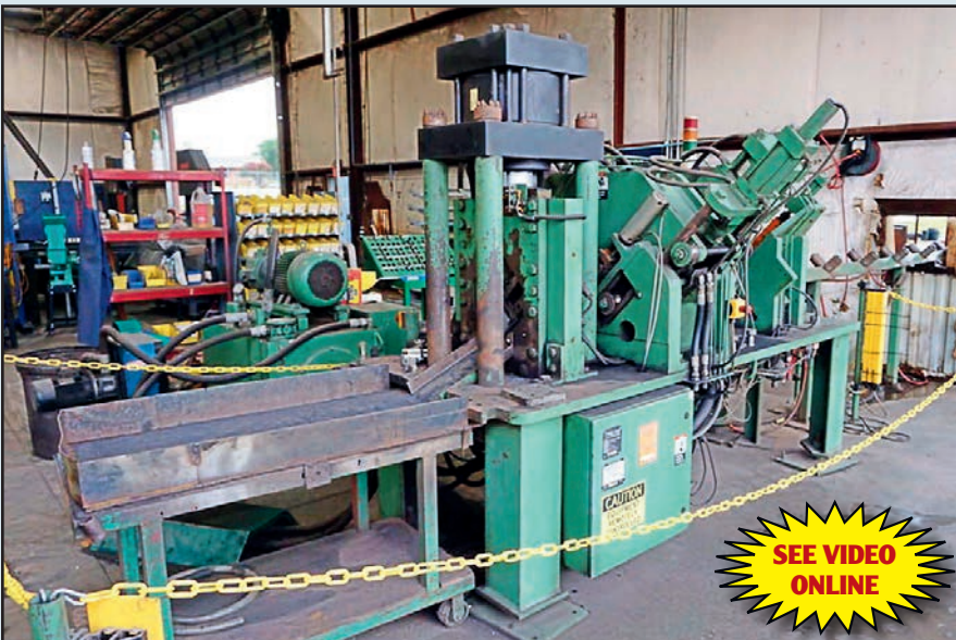
PEDDINGHAUS ANGLEMASTER 643 ANGLE LINE, 6" X 6" X 5/8", 75-TON PUNCH CAP., 230-TON SHEAR CAP.
