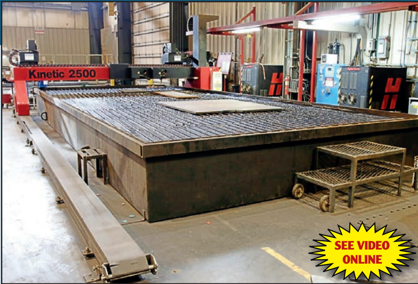
2006 KINETIC MDL. K2500-DA 2,500-WATT CNC PLASMA CUTTING TABLE, 120" X 480" CUTTING CAP., EST. 20' X 50' WORKTABLE WITH (2) HYPER THERM MDL. HPR260 PLASMA CUTTING UNITS, THERMCO MDL. 6105CA30A1100 GAS MIXTURE, S/N 28266, ASSET #000239, (2008), 0-2,000 SCFH CAP., THERMCO MDL. 6105CA30A1175 GAS MIXTURE, S/N 17682, (2013), 0-2,410 SCFH CAP., (LOCATED: 850 AEROPAZA DRIVE, COLORADO SPRINGS, CO).
