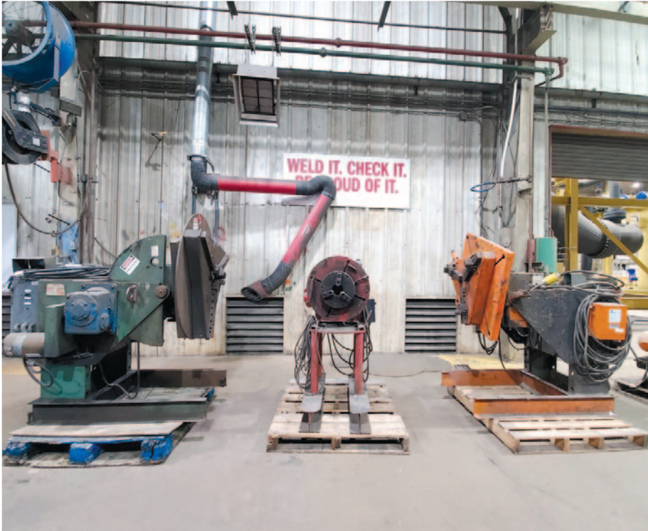
• View of Welding Positioners
