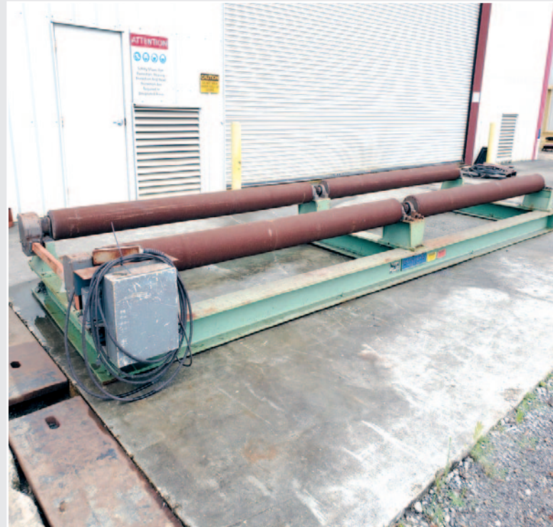
• View of Welding Fitup Rolls
