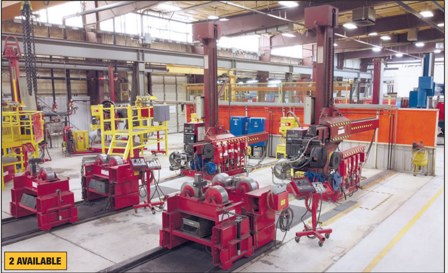
VIEW OF WELDWARE SUB ARC WELDERS, (2) TURNING ROLLS WITH LINCOLN POWERWAVE AC/DC 1000 POWER SOURCE AND WELD ENGINEERING MM-3000 FLUX RECOVERY VACUUM AND DUST COLLECTOR
