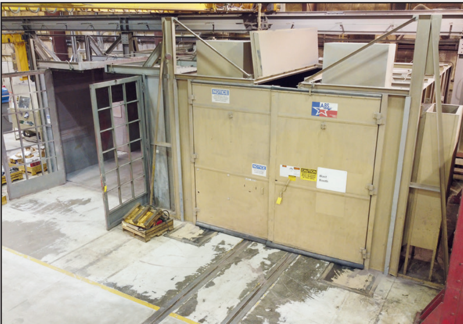
VIEW OF PAINT BOOTH, 18'D. X 16'W. X 14'T. AND ABS BLAST BOOTH, 22'D. X 17'W. X 14'T.
