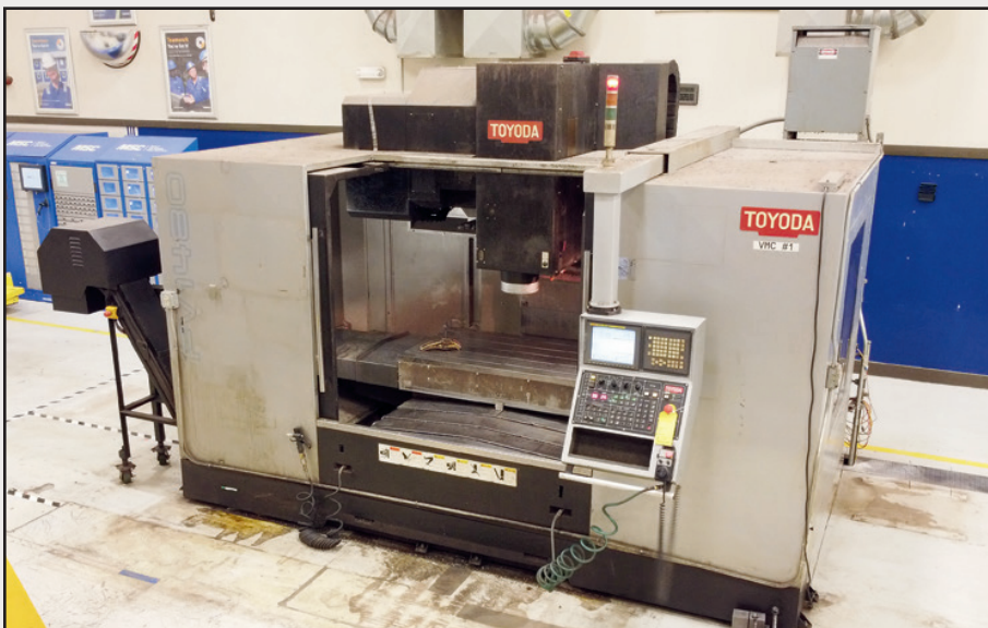
TOYODA FV-1480 VERTICAL MACHINING CENTER, X-AXIS TRAVEL 55", Y-AXIS TRAVEL 31", Z-AXIS TRAVEL 27", FANUC 18i MB CONTROL, 50 TOOL TAPER, MAX. SPINDLE SPEED 6,000, 30 ATC, WITH CHIP CONVEYOR.
