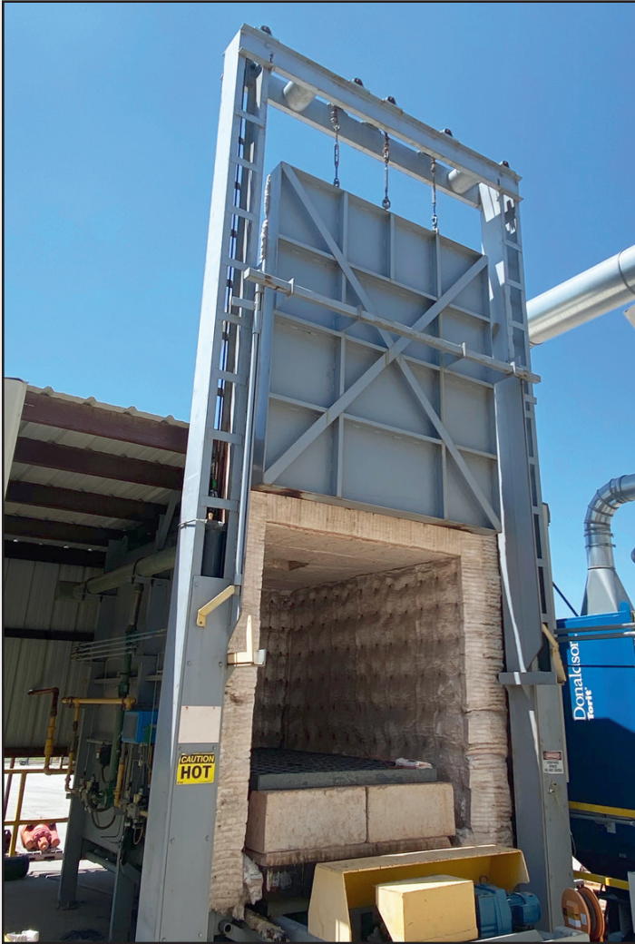
BLAGRAVE & DUFFEY 1,850 DEGREE GAS STRESS RELIEVING FURNACE
