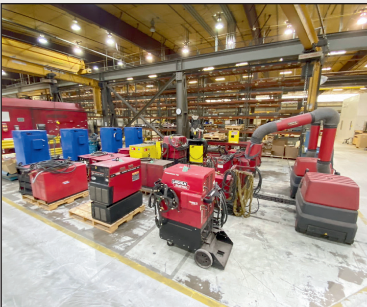
VIEW OF LINCOLN WELDERS AND FUME COLLECTION
