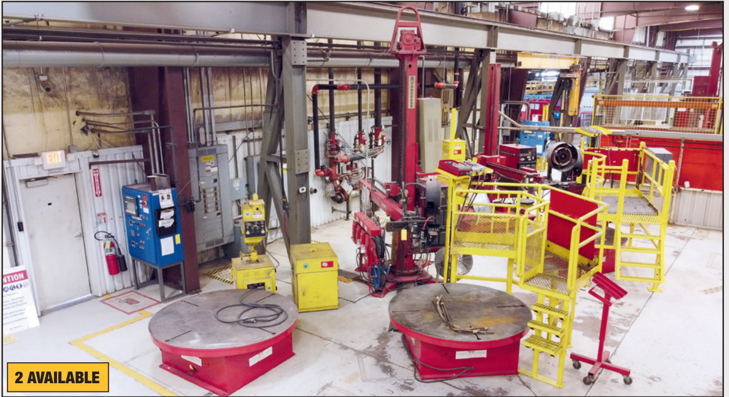
VIEW OF WELDWARE SUB ARC WELDERS, (2) POSITIONERS WITH LINCOLN POWERWAVE AC/DC 1000 POWER SOURCE AND WELD ENGINEERING MM-3000 FLUX RECOVERY VACUUM AND DUST COLLECTOR
