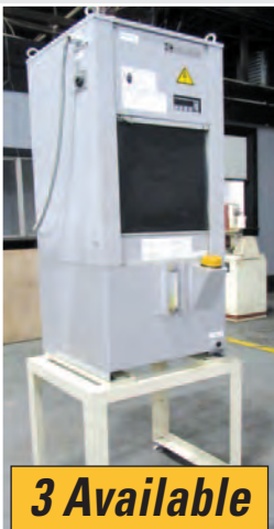
• Kanto Seiki MPSB-07-N Auto Oil Chiller, 7.5/0.75kw, R-407C refrigerant (950g)
