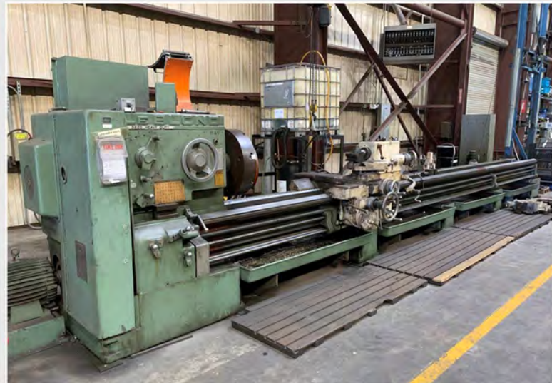
• 32" x 312" LeBlond 3220 HD Engine Lathe, 32" swing, 20.5" over cross slide, 312" centers, 10 - 1300 rpm, 30 hp, threading, 24" 4-jaw chuck, tailstock, steady rests, Aloris tool post
