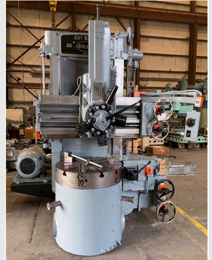
• 36" Bullard Cutmaster VTL, 36" tbl, 45" swing, 30" under rail, 3.3 - 240 rpm, 30 hp, swivel turret head, side head
