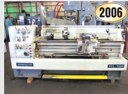
• 16" x 60" Birmingham YCL-1660 Gap Bed Engine Lathe , 2006, 25-2000 rpm, 7.5 hp, 2.28" bore, threading, (2) chucks, tailstock
