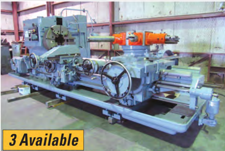
• Warner & Swasey Model M-3600 Square Head Saddle Type Turret Lathe, with Cross Sliding Rear Turret, 36.5" swing, 83" max. turn length, 12.5" bore, 10-281 rpm, 75 hp, 32" chuck, 6 pos. rear turret, 4-way tool post
