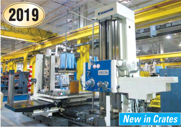
• 5" KMT MB130e HBM, New 2019, 5.11" spindle, #50 taper, 8-900 rpm, 20 hp, 63" x 70.8" table, 78.7" X, 74.8" long. trvl, 78.7" headstock vert. trvl, built-in facing head
