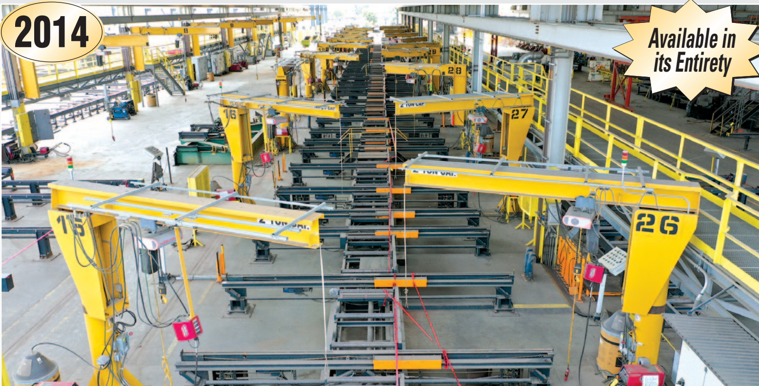
Welding Bay: 2014 Ficep Material Handling System
