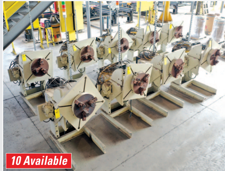
View of Pandjiris Welding Positioners with Power Tilt and Power Turn
