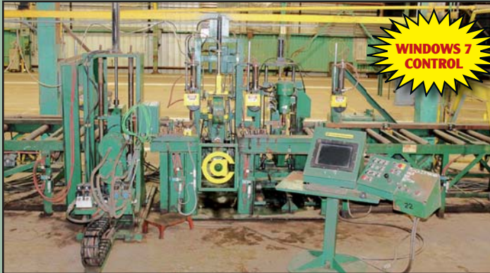
CONTROLLED AUTOMATION Beam Punch Line , 5-station, top flange, bottom flange and web punch, min. width 6", max. width 36", 3/4" max. thickness, 75' infeed conveyor, 60' outfeed conveyor, 52" width, (4) 20' transfers.
