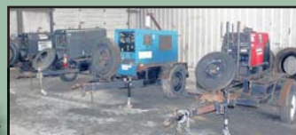
(3) Portable Welders, trailer mounted.
