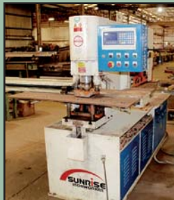
2012 SUNRISE CNC Ironworker, 110-ton, w/CNC back gauge.
