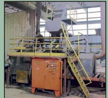
Pass-Through Beam Blast System, w/dust collector and recycle system, 35' infeed conveyor, 40' outfeed conveyor, 52" width, 4' wide, 3' tall opening.
