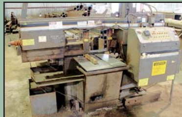
HEM H105A Horizontal Bandsaw, 27" max. cut width.
