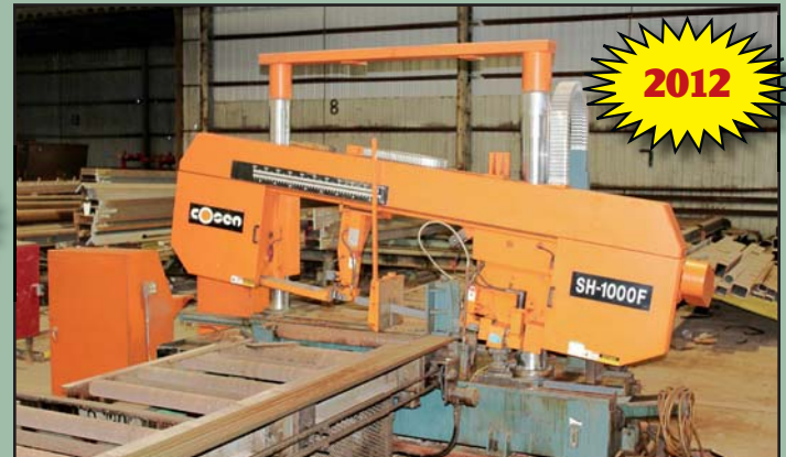
2012 COSEN SH-100F Dual-Column Horizontal Bandsaw , max. width 40", w/chip removal system, 60' infeed conveyor, 62' outfeed conveyor, 52" width, (9) 27' transfers.
