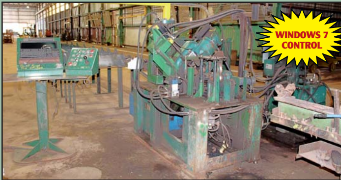
CONTROLLED AUTOMATION 6x6 Angle Line , 6" x 6" x 3/8".
